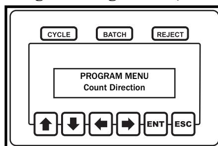
This unit can be programmed to count up from zero until the batch is reached or count down from the batch to zero.
