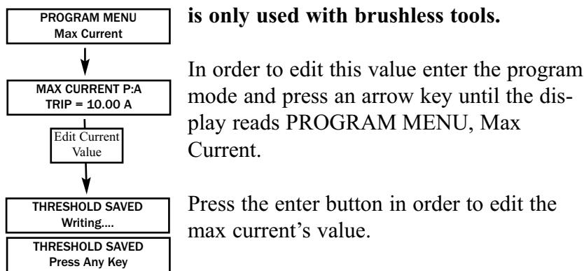
In order to edit this value enter the program mode and press an arrow key until the display reads PROGRAM MENU, Max Current.
