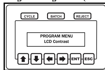
The LCD display can be adjusted so that the text is darker or lighter by accessing the LCD Contrast feature.
