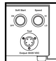
A five pin circular connector is located on the face of the unit. This connector is used to supply power to a tool and also to read signals back from the tool.
