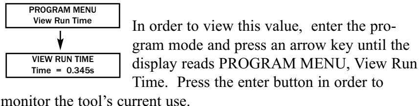
In order to view this value, enter the program mode and press an arrow key until the display reads PROGRAM MENU, View Run Time. Press the enter button in order to monitor the tool’s current use.
