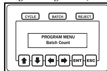
The Batch Count is typically programmed to be the number of fasteners in a given assembly. A Cycle Accept signal will be generated each time a proper fastening occurs. A Batch Accept however, will occur when the count reaches the
