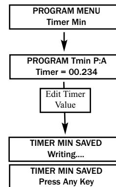
In order to edit this value enter the program mode and press an arrow key until the display reads PROGRAM MENU, Timer Min.
