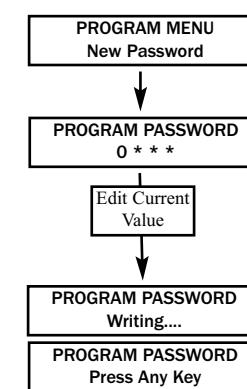
In order to change the password, enter the program mode and press an arrow key until the display reads PROGRAM MENU, New Password. Press the enter button in order to edit the password.
