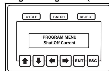
The shut-off current defines the minimum amount of current that needs to be drawn by a brushless tool when the tool clutches out. This threshold can be used as a secondary check for the tool's clutch setting. **The shut-off current**
