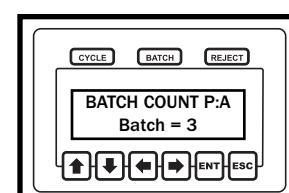
**Step 7:** Use the up and down arrows to modify the batch count by one. The left and right arrows modify this value by 10 in either direction (up or down).
