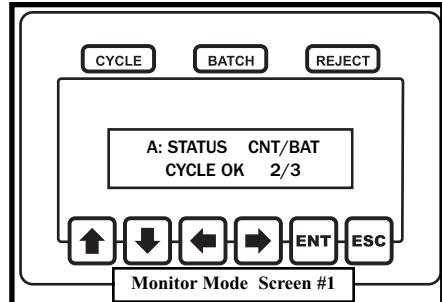
The first of these screens will show the current parameter, status of the last fastening, current count and the number of fasteners in the batch.
