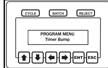
The bump timer defines an amount of time that a tool can run and that run will be ignored if the clutch does not fire (i.e. torque is not achieved). This timer may be used to eliminate nuisance rejects.
