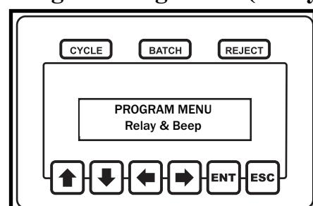
The output relays in this system can be programmed to be either momentary or latching. If the relays are momentary the will close briefly (200ms) when an event occurs. When set to latching, the relay closes and remains that way until the
