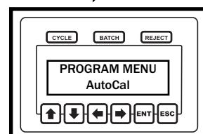
**Step 4:** Use the arrow keys to navigate to the AutoCal option on the program menu. Once at the AutoCal option, press the enter (ENT) button to select it.
