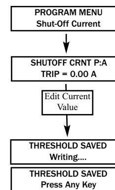
In order to edit this value enter the program mode and press an arrow key until the display reads PROGRAM MENU, Shut-Off Current.
