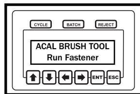
**Step 5:** The display will ask for a fastener to be run. Run the tool on the target fastener allowing the clutch to turn the tool off. After the clutch fires, the display should read AUTOCAL COMPLETE Press Any Key.
