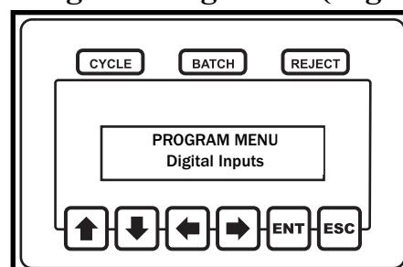
The Digital Inputs menu option is a trouble shooting mode. If this item is selected, the signals that the tool is sending the TS-III can be monitored.
