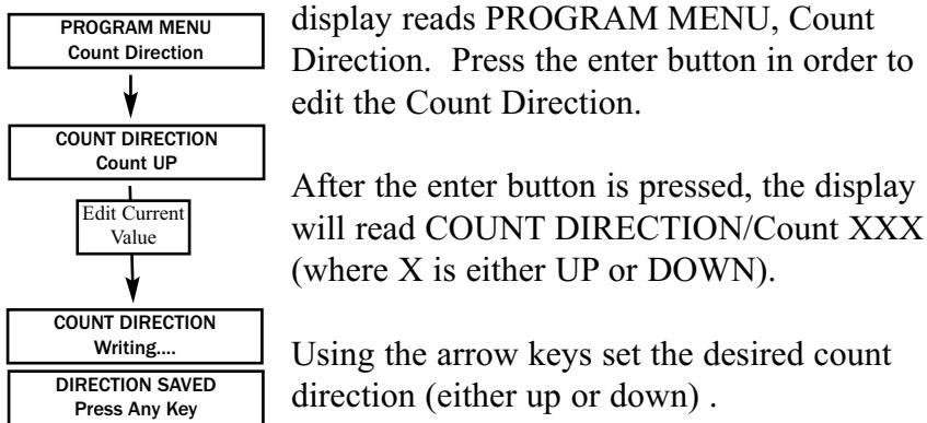
After the enter button is pressed, the display will read COUNT DIRECTION/Count XXX (where X is either UP or DOWN).
