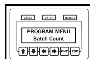
**Step 6:** Use the arrow keys to navigate to the Batch Count option on the program menu. Once at the Batch Count option press the enter (ENT) button.
