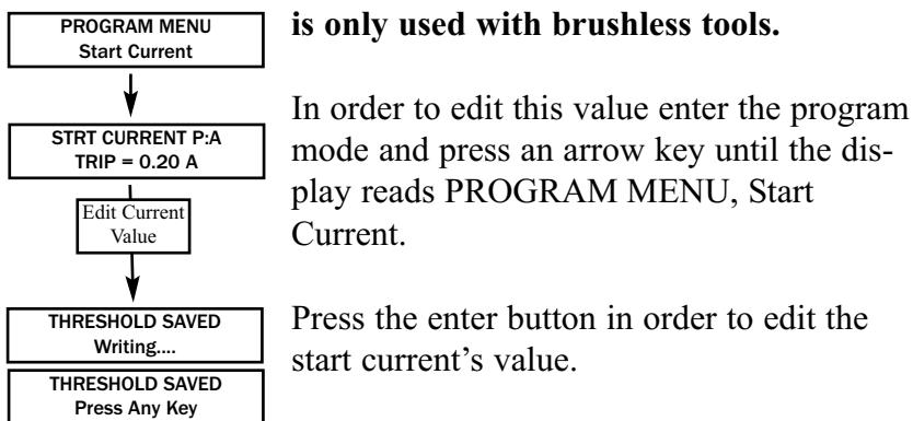
In order to edit this value enter the program mode and press an arrow key until the display reads PROGRAM MENU, Start Current.
