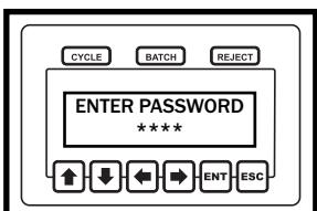
**Step 3:** Press the enter (ENT) button and enter the programming mode. Either enter the password (0104 default) or bypass the password by using the key.
