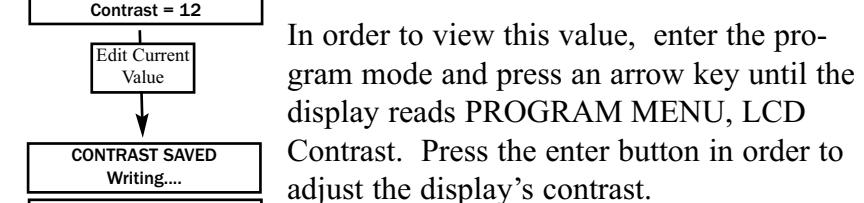
In order to view this value, enter the program mode and press an arrow key until the display reads PROGRAM MENU, LCD Contrast. Press the enter button in order to adjust the display’s contrast.
