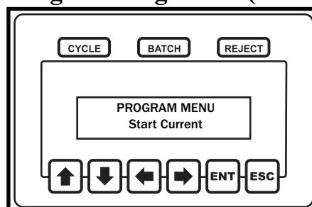
The start current defines the amount of current that needs to be drawn by a brushless tool before the unit is considered to be in cycle. Once the tool starts drawing this amount of current, the run-timers will start. **The start current value**
