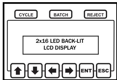
A two line by sixteen character back-lit LCD display is part of the user interface. This display will provide the user with feedback during the run mode and guide the user through programming functions.
