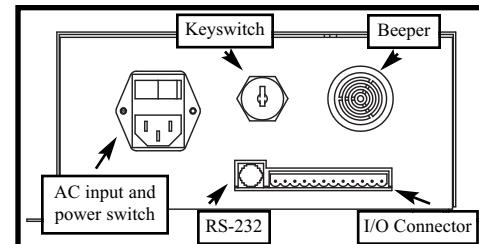
The rear panel on the unit contains several items. The main power switch for the unit and the power entry module are found on the back panel. This unit is capable of running on an AC input voltage of 100VAC to 240VAC.
