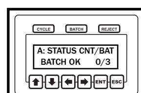
**Step 8:** Pressing the escape (ESC) key several times will return the unit to the main run screens.
