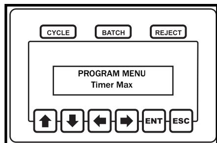
The maximum run timer defines the maximum amount of time a tool can run during a fastening process and still be considered a good fastening. If a fastening takes longer than timer max, a Tmax reject will be issued.
