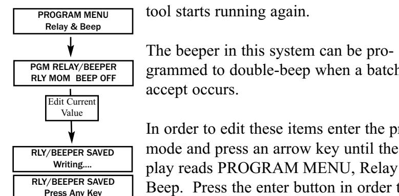
In order to edit these items enter the program mode and press an arrow key until the display reads PROGRAM MENU, Relay & Beep. Press the enter button in order to edit relay or beeper settings.
