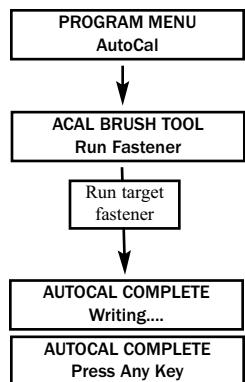
The display will read ACAL BRUSH TOOL or ACAL B-LESS TOOL and Run Fastener. Be sure that the right type of tool is being used with the unit before proceeding.
