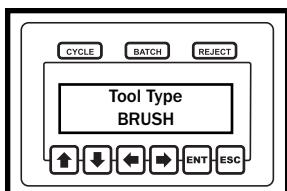
**Step 1:** Power up the unit. During power-up the device will identify the tool type for which the unit is configured (either Brush or Brushless). Be sure that the tool to be used with this device matches the tool type.
