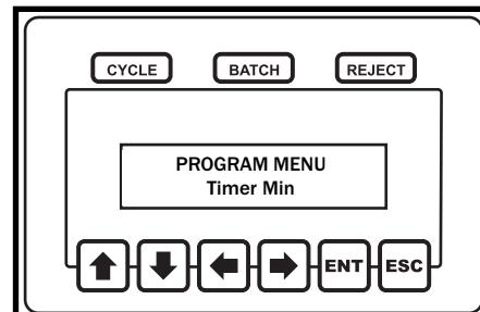
The minimum run timer defines the minimum amount of time a tool has to run during a fastening process in order to be considered a good fastening. If a fastening process is shorter than timer min, a Tmin reject will be issued.
