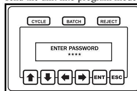
If the keyswitch is in the locked position, the user will be prompted to enter a password before continuing.
