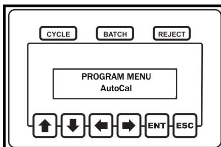
The first item on the program menu is AutoCal<sup>TM</sup>. AutoCal is a calibration routine that is meant to get the unit up and running very quickly. In order to use the AutoCal<sup>TM</sup> feature press the enter button.
