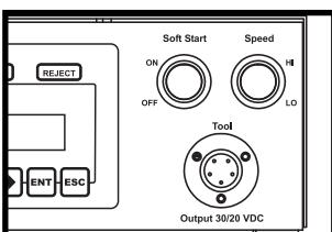
**Step 2:** Plug the into the tool connector. Select the desired tool speed (HI or LO). Turn the Soft Start either ON or OFF.
